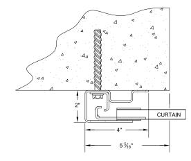
USING 1/4-14 X 1" SELF-DRILLING SCREW
